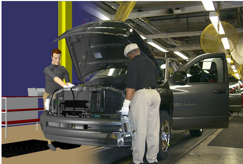
Graphic 5: Virtual Ergonomic Simulation Created by DELMIA Digital Manufacturing Solutions Source: Courtesy of Dodge Truck Advanced Design & Packaging Group
