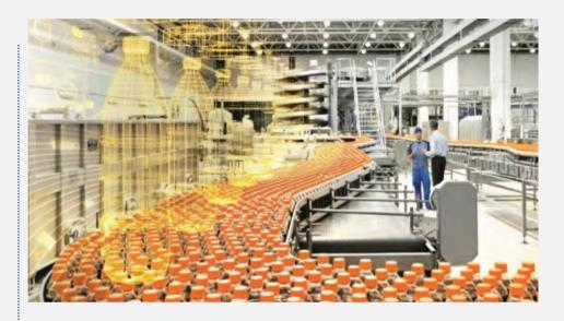
The digital twin is a virtual model of a physical item. The model represents a specific product, configuration, piece of equipment, plant, city, or other physical asset with enough fidelity to simulate, validate, and optimize performance and behavior.
